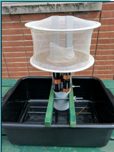
Traps – these were placed in order to trap mosquitos and send to the ODH Lab for testing. This surveillance aids the GCHD in determining whether mosquitos are carrying certain diseases in the Galion area.
